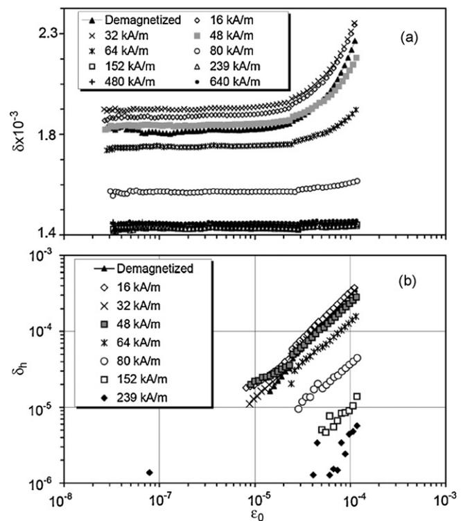
Fig. 2. Strain amplitude dependence of the total internal friction  $\delta$  (a), and its amplitude-dependent component  $\delta_h$  (b), for a Ni–21.5Fe–27Ga (at.%) single crystal at room temperature ( $T=300$  K, austenite), under different transverse polarizing fields up to 796 kA/m.
