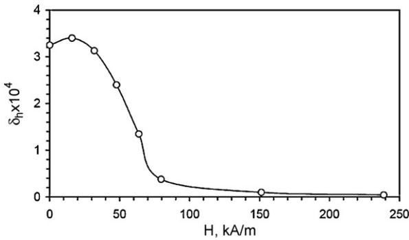
**Fig. 3.** Amplitude-dependent internal friction ( $\delta_h$ ) for a Ni-21.5Fe-27Ga (at.%) single crystal, as a function of transverse polarizing field, at room temperature ( $T=300$  K, austenite).
