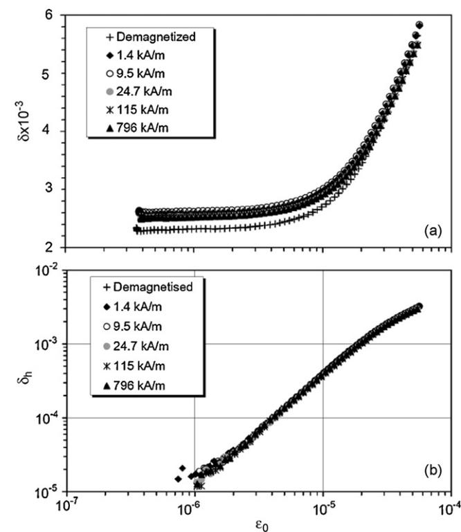
Fig. 1. Strain amplitude dependence of the total internal friction  $\delta$  (a), and its amplitude-dependent component  $\delta_h$  (b), for a Ni–19Fe–27Ga (at.%) polycrystal at room temperature ( $T=293$  K, austenite), under different transverse polarizing fields up to 796 kA/m.
