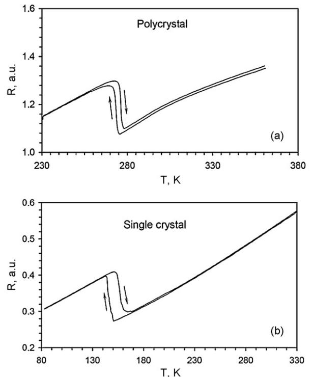
**Fig. 5.** Resistance in a cooling-heating cycle through the martensitic transformation, for both poly (a) and single (b) crystals of Ni-Fe-Ga alloys.
